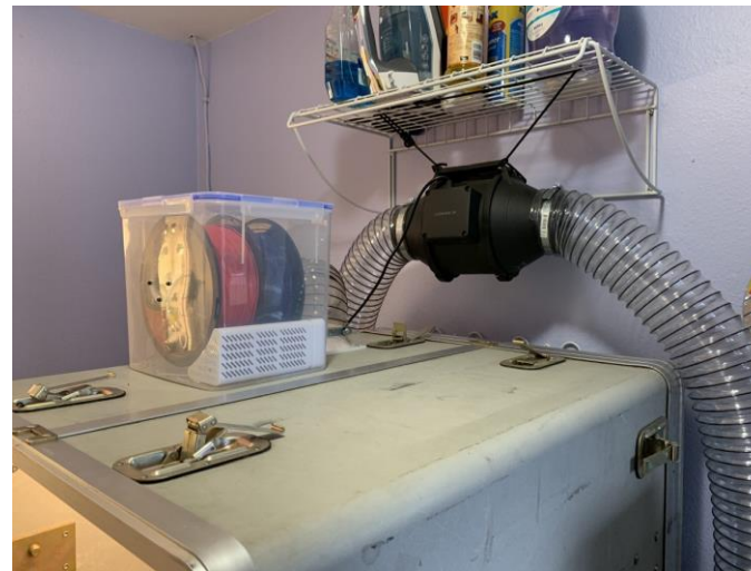
Quiet DC exhaust fan, suspended to mute vibrations
